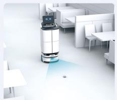
The robot, outfitted with three RGBD cameras and LiDAR, can precisely identify obstacles and individuals, enabling it to reach its destination safely and seamlessly even in tight spaces.
